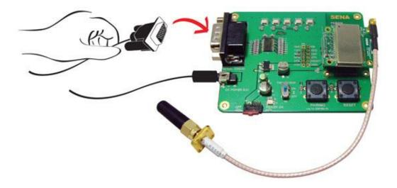
Figure 2-4 Connecting a Device to Development Board
