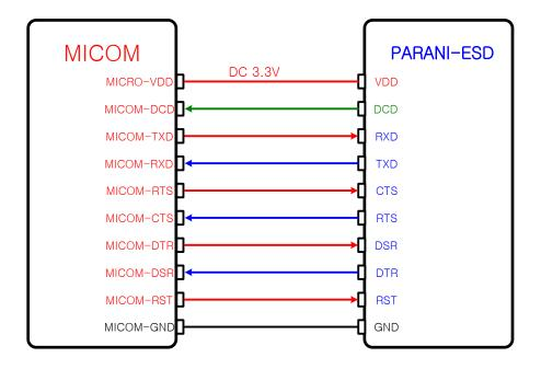
A.2.1.2. When TTL level of MICOM is 3.3V and Hardware Flow Control is not used
