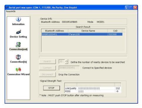
Figure 3-7 Signal Strength Test
