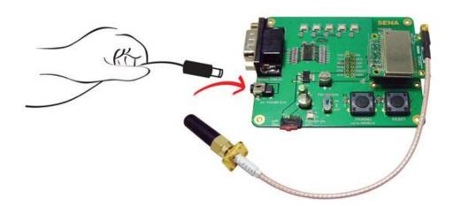
Figure 2-3 Connecting Power to Development Board
