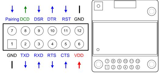
Figure A-1 Pin Assignment of Parani-ESD
