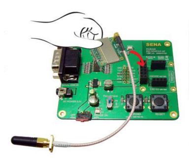
Figure 2-2 Connecting Parani-ESD to Development Board
